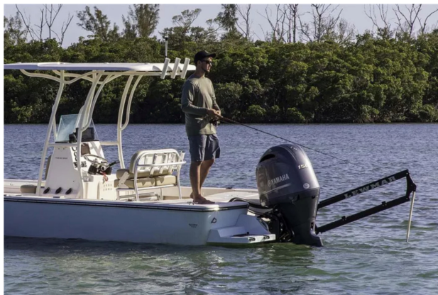
Lewmar's Axis shallow-water anchor eliminates the need for hydraulic pumps and supply hoses.
